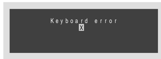
Fig. A.4 — Error screen, depressed key during start-up.
